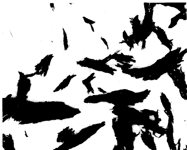
Figure 21 Transmission electron microscopy of urea-terminated poly(1,6-hexamethyleneurea) particles isolated from a polyurea polyol dispersion
